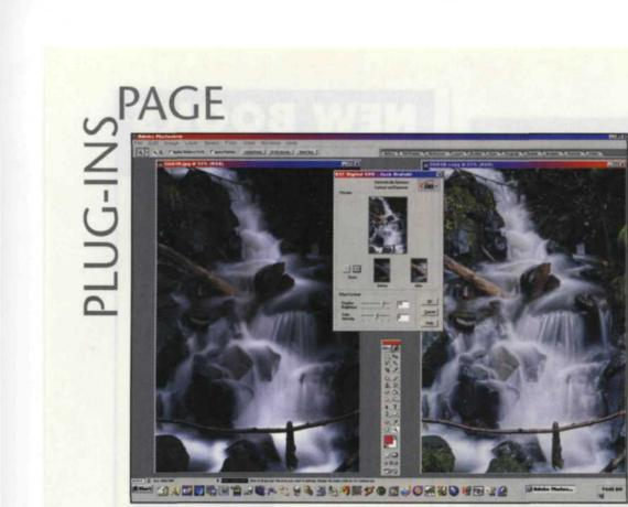
Applied Science Fiction Digital SHO plug-in filter for Adobe Photoshop. Menu shows before and after filter, zoom in and adjustments to shadow brightness and color intensity. Before image on left...after image on right.
